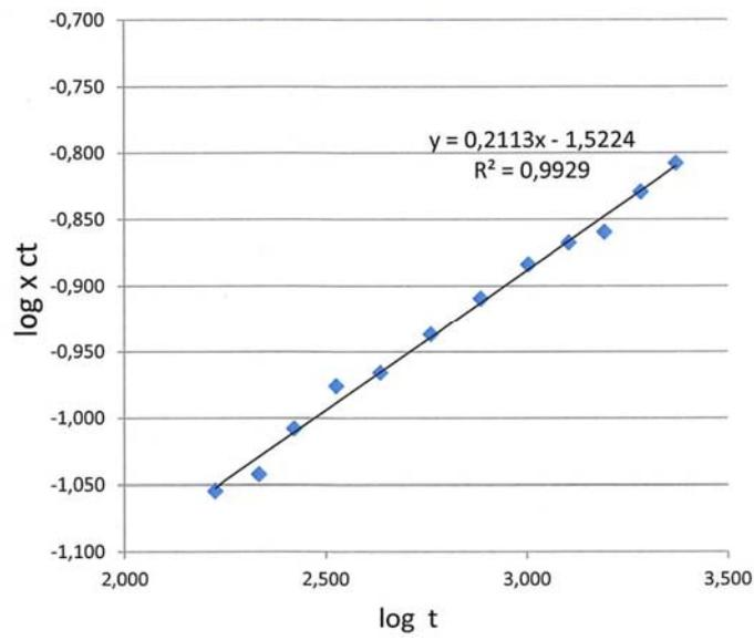
Figure 3.2 Regression analysis of the compressive creep of product AK300HT
