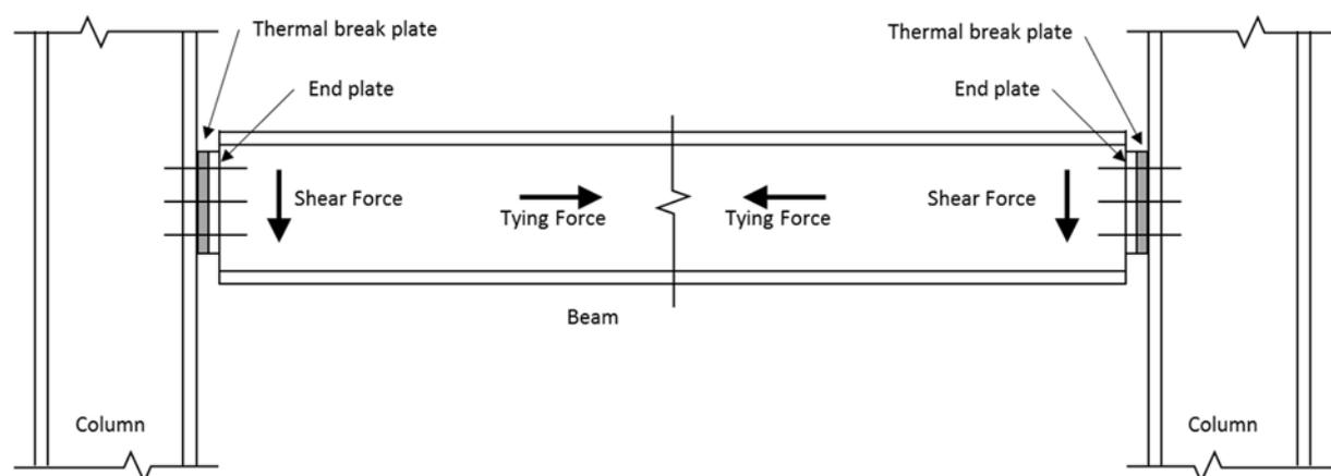
**Figure 4.1 Nominally pinned connection with thermal break plate**
