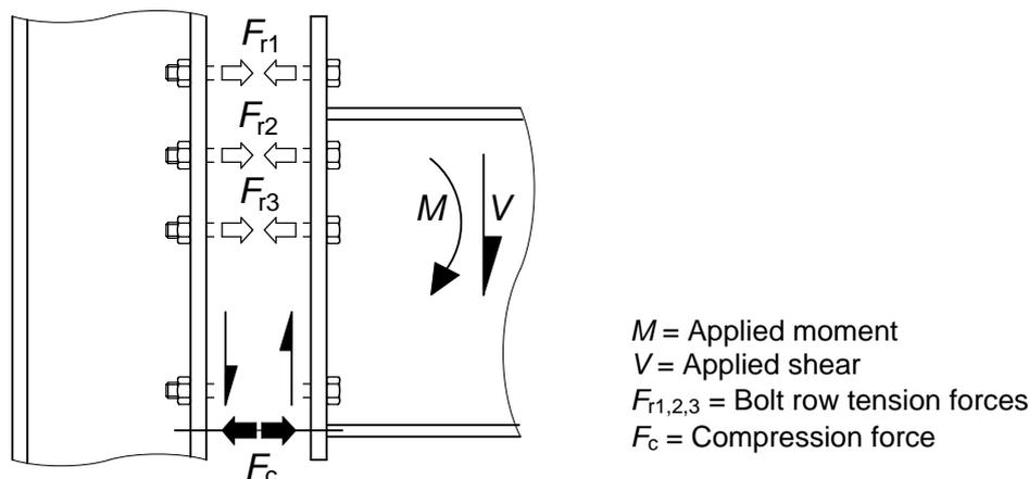
**Figure 4.2 Forces in a typical moment connection**
