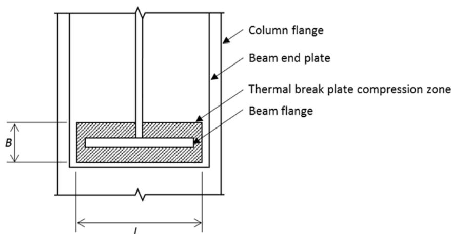
Figure 4.4 Thermal break plate compression zone
