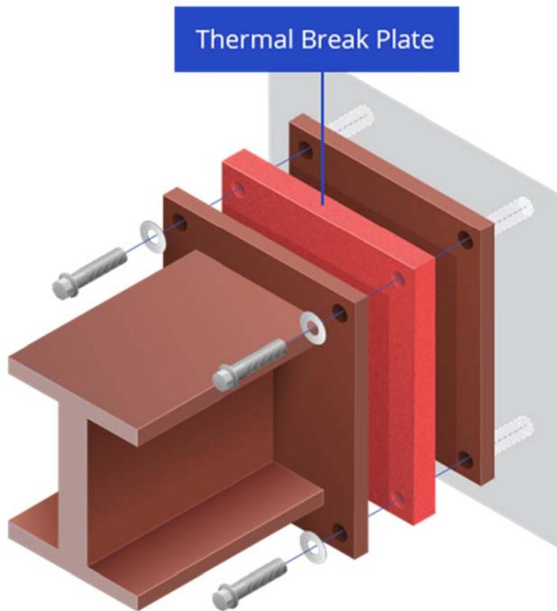
Shows Steel to Concrete connection
