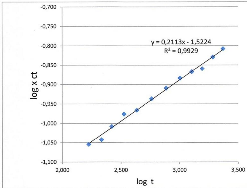
Figure 2: Regression Analysis of the compressive creep behavior of the Material „AK300HT“
