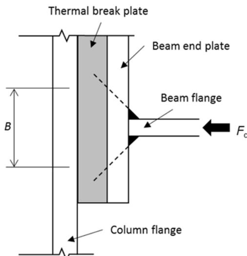
Figure 4.3 Dispersion of force through connection compression zone
