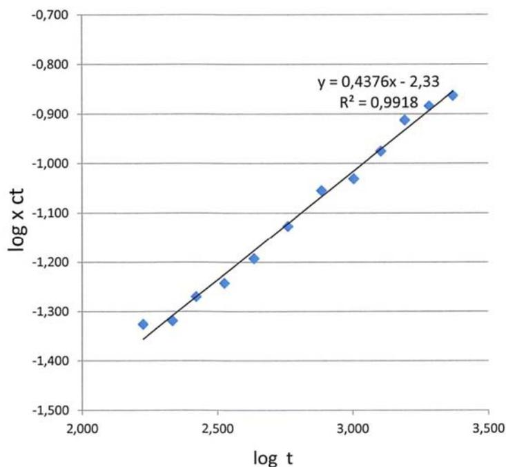
**Figure 3.1 Regression analysis of the compressive creep of product AK200**
