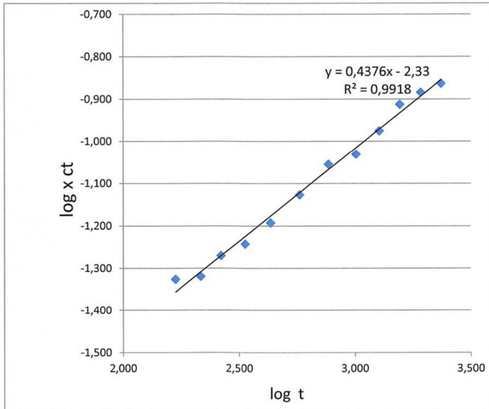
Figure 1: Regression Analysis of the compressive creep behavior of the Material „AK200“
