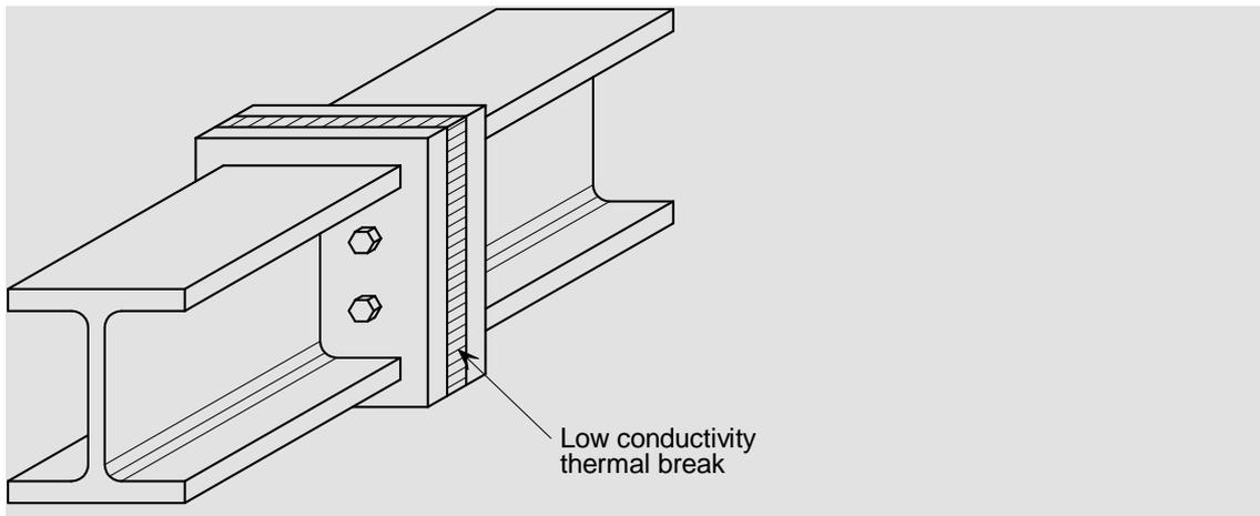
**Figure 1.1 Thermal break between steel beams**
